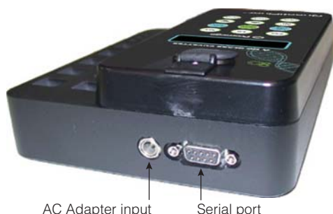
Figure 2. Top view of the QuantiFluor™-ST Fluorometer showing the AC Adapter Input.
