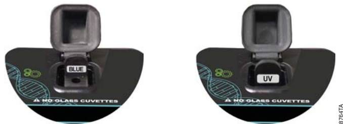
Figure 5. Inserting the QuantiFluor™-ST Minicell Adapter.
