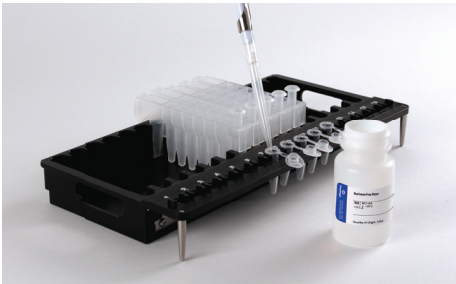
Figure 2. Setup and configuration of the deck tray. Nuclease-Free Water is added to the Elution Tubes as indicated.
