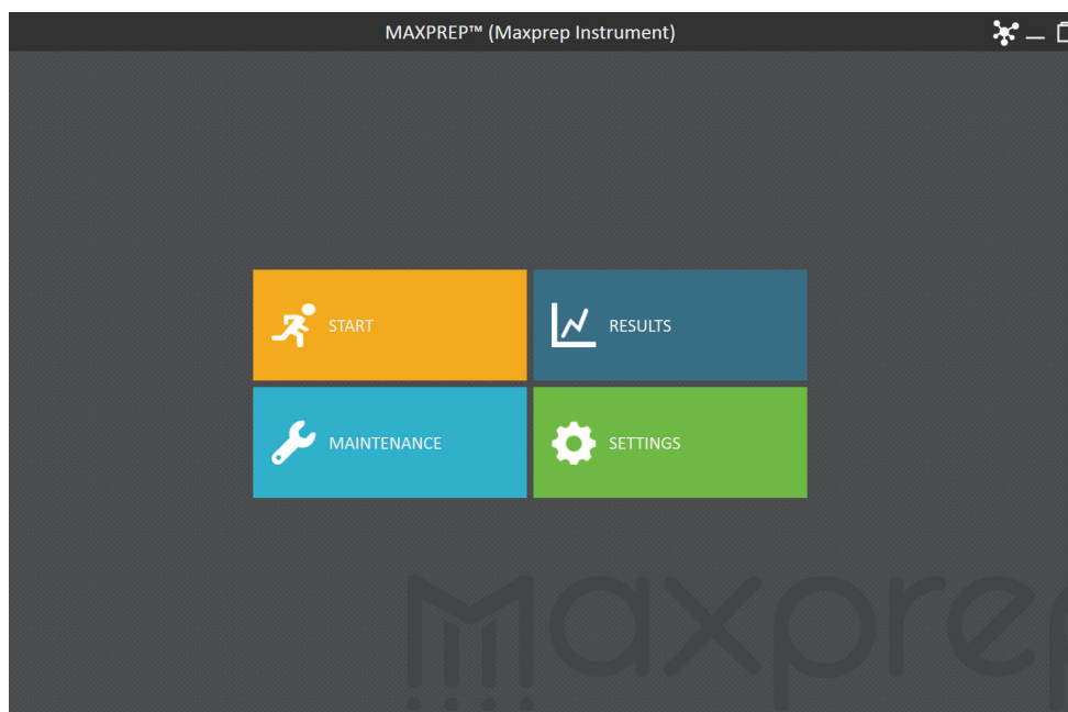
Figure 1. Maxprep™ software 'Home' screen. From the Maxprep™ software 'Home' screen, select the Start button to begin running a method.
