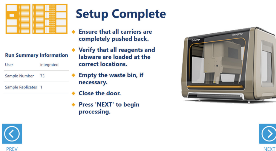
Figure 13. Final instrument setup screen. This screen presents a list of items that should be checked before starting automated processing. It also provides a final chance to return to any of the previous instrument setup screens before automated processing begins. To start processing, close the instrument door and press the Next button.
