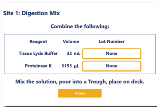
Figure 2. Reagent Detail pop up screen for the Digestion Mix. The details window will specify how much volume of Tissue Lysis Buffer or Proteinase K (in ml or µl, respectively) to combine and place in a trough.
